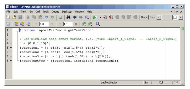
Once this function is saved as GETTESTVECTOR, you can create a SystemTest test vector whose expression is set to GETTESTVECTOR. This will create a 1-by-3 test vector cell array within the SystemTest software, where each entry in the cell array represents the time and signal data for the three Inport blocks.
